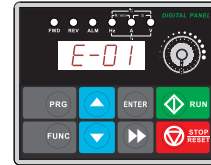
Fault alarm display of over current during accelerating
